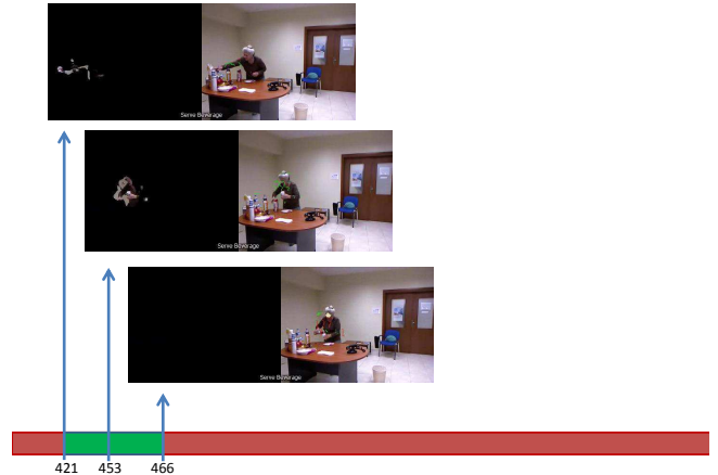
Figure 2: Activity detection throughout a video. Activity Areas are depicted on the left of each frame while on the right trajectories are depicted. Green trajectories are active, while red are the terminated ones.
